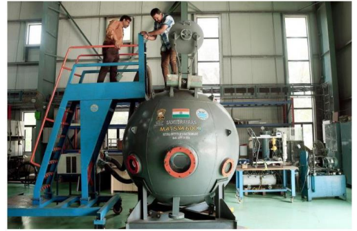
A prototype of the MATSYA 6000, a submersible made by the National Institute of Ocean Technology in Chennai. The final version is expected to undertake a journey to a depth of 6,000 metres. R. RAVICHANDRAN
